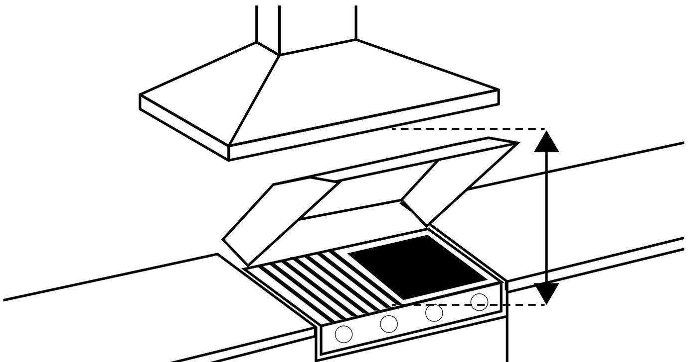
Measurements are from the top of the trivets to the lowest part of the rangehood, including the button controls.
