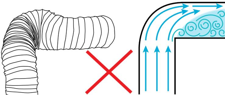
1. Crushed or kinked ducting creates sharp corners that creates turbulence. This reduces the size and efficiency of the ducting, lowers extraction and may cause excessive noise.
