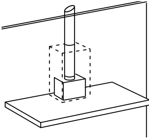
Straight ducting is the most effective installation
