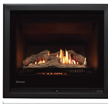
Rinnai 750 740mm wide 6kW heat output 27mj/h gas input
