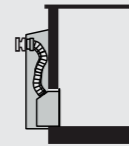
Weather Proof Box Reduces the internal footprint requirements of the heater engine
